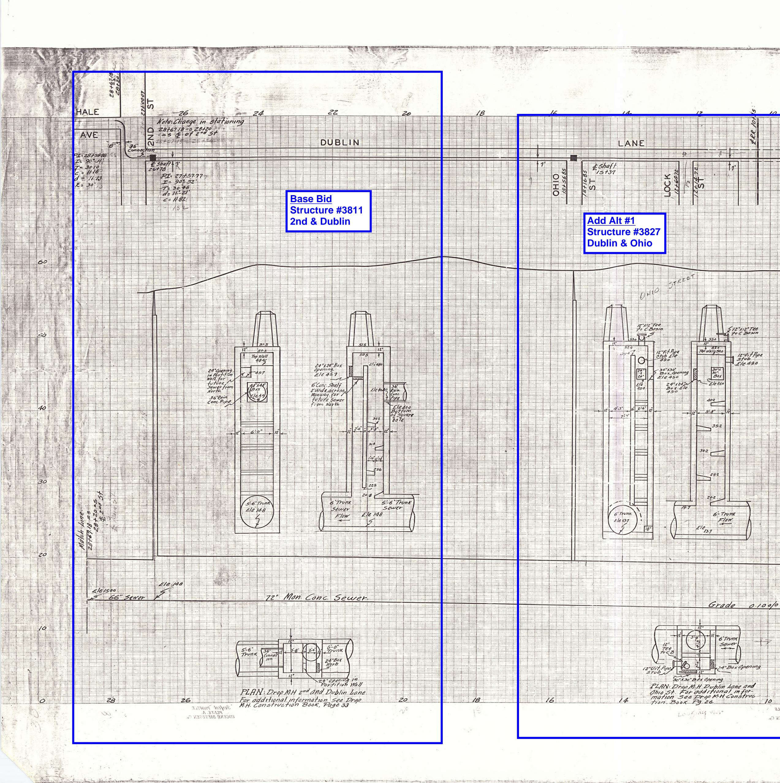
**1. Record Drawings are provided only as a reference for understanding of general** manhole depths and layouts. RWRA cannot guarantee accuracy. Contractor shall field verify any dimensions or layouts required prior to work.
