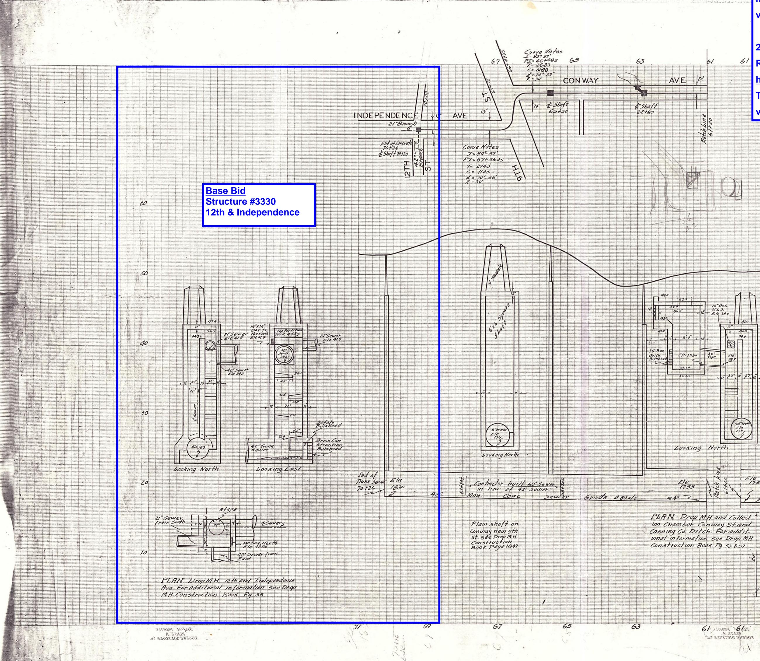
**1. Record Drawings are provided only as a reference for understanding of general** manhole depths and layouts. RWRA cannot guarantee accuracy. Contractor shall field verify any dimensions or layouts required prior to work.
